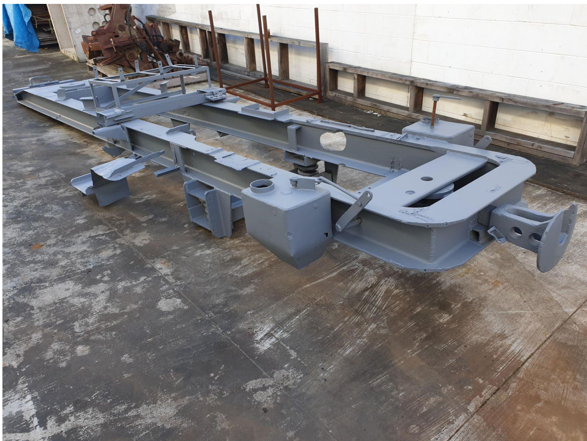
The 5 axle rail truck chassis recently seen at Ian Jenners' workshop in Auckland (Photo: I. Jenner)
