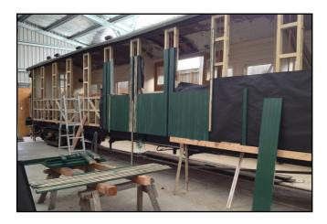
Work continues on this. Bob has painted more tongue and groove, some of which has been nailed onto the car. Robin has started cutting some of the window sills to size.
