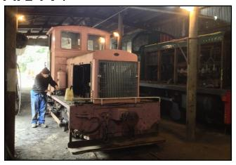
This loco has not been used for a couple of years because of a bad limp in the drive to the wheels. Mike spent three days getting the motor going and is presently looking at the axle bearing oil boxes. This was a very useful loco some years ago.
