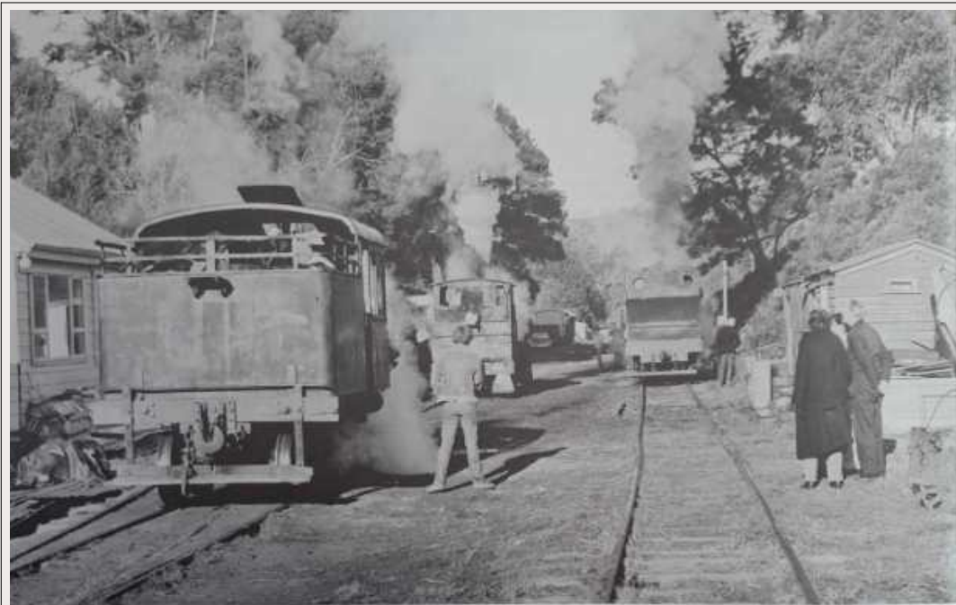
ABOVE: Getting ready for "Open Day" on 17 May 1981 at Pukemiro during National Rail History Week, members of the Bush Tramway Club are busy raising steam on three steam locomotives. From the left you will recognise the Heisler (ready and waiting to go), the "F" 0-6-0T No.185, and the Peckett. The "F" is taking on coal, and the Peckett is taking on water. The 1982 "Rail History Festival" will extend from 10 May to 21 May with most activity concentrated on the weekend of 15 and 16 May.
