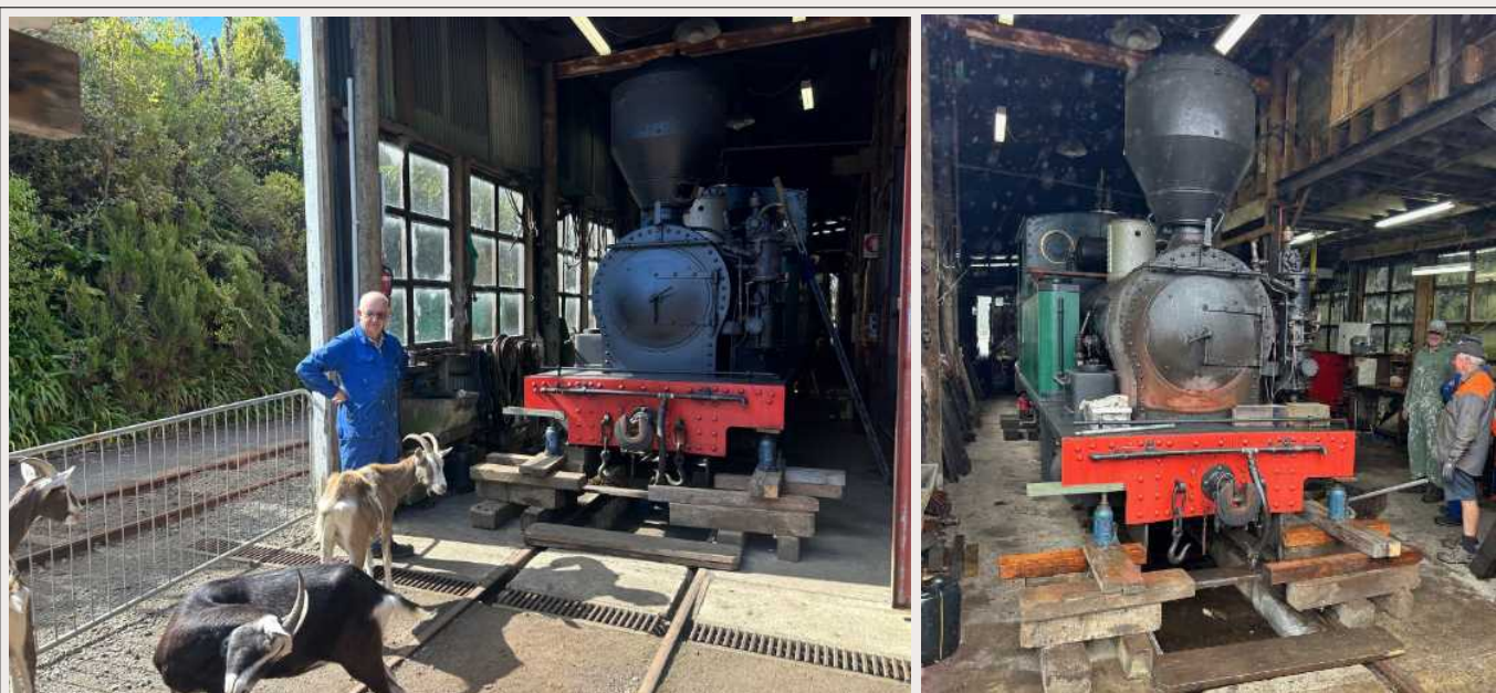
Above: The Peckett is on blocks during annual boiler survey for ancillary work on axle bearing & a broken leaf spring (Chris M)
