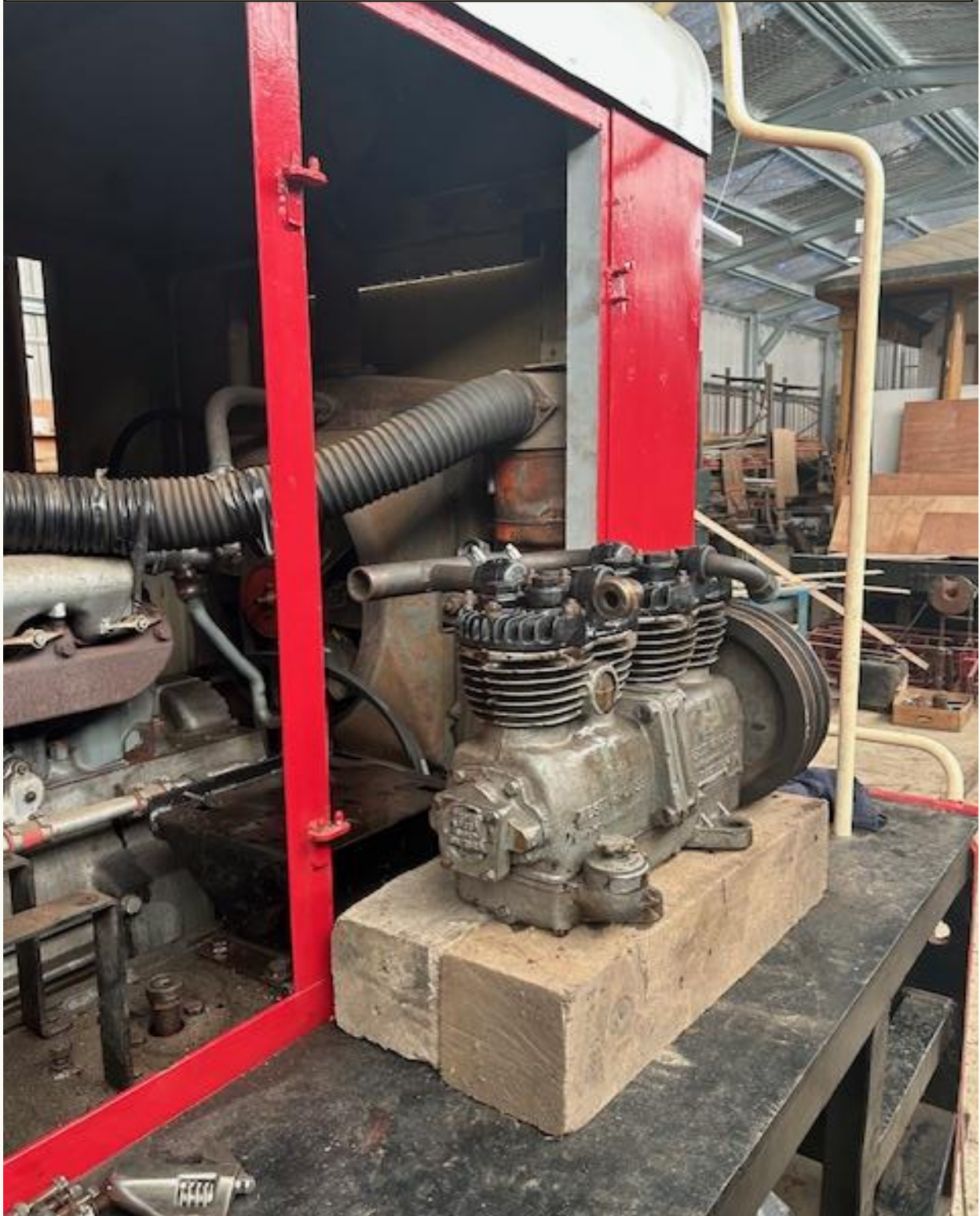
Compressor for Tr105 before re-installation (Chris M)
