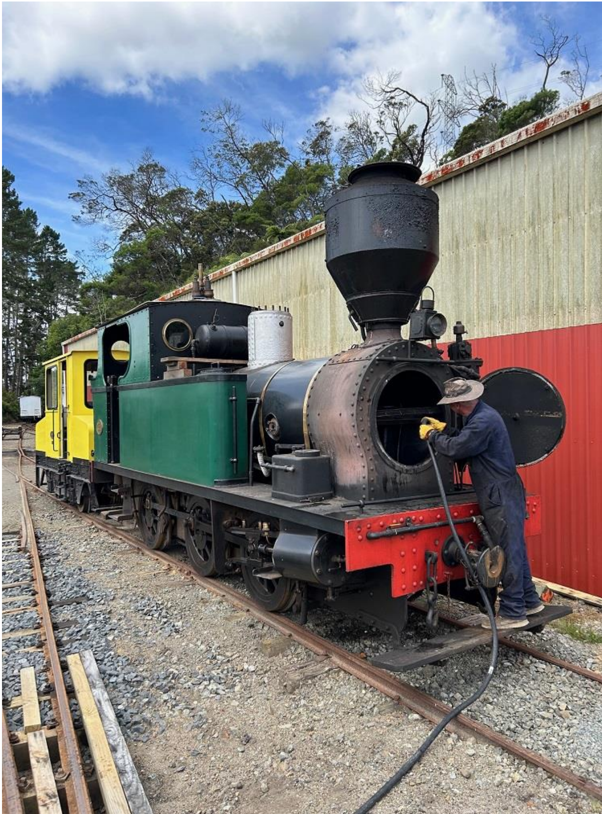
The Peckett being stripped for inspection, J. Soffe cleans the smokebox (C. Mann)
