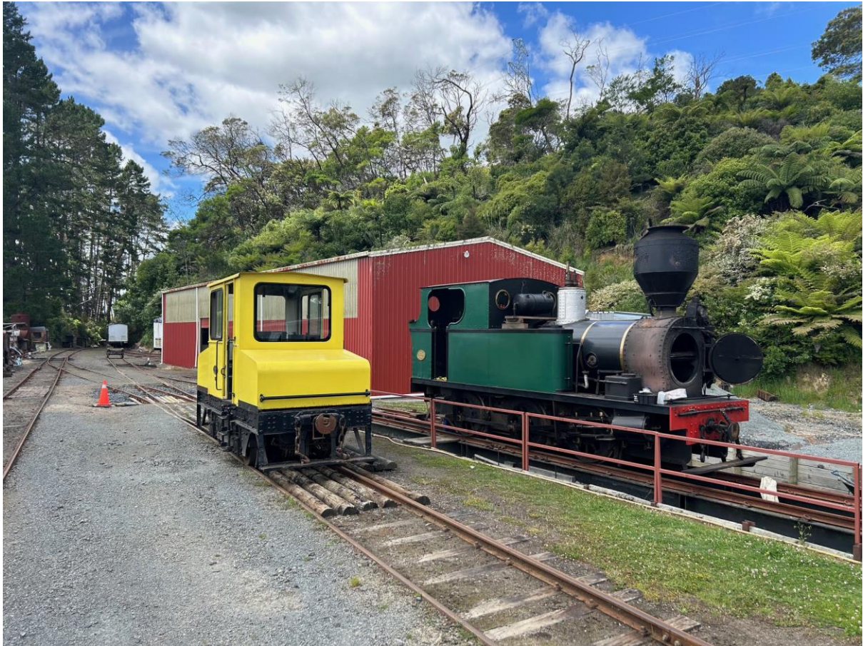
The battery electric loco and the Peckett which was being prepared for its annual inspection at the time (C.Mann)
