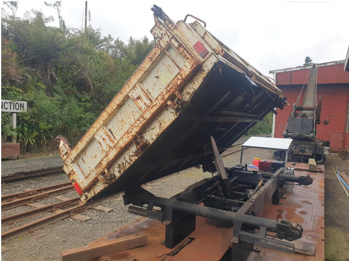
The Isuzu tipper body mounted on the old Huntly West mine wagon (LJenner)
