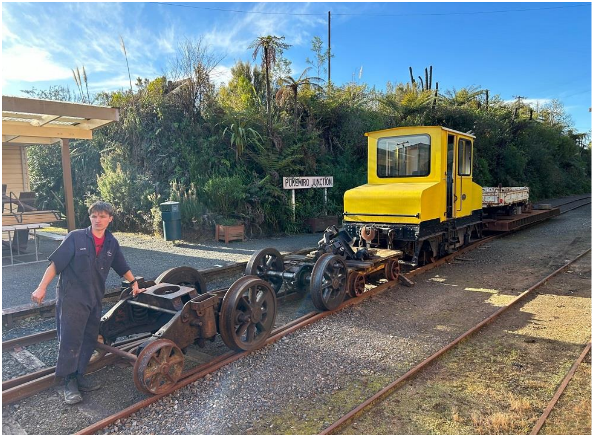
Heisler bogies, the battery electric loco, the new tipper wagon setup and BTC member Evan W (C.Mann)
