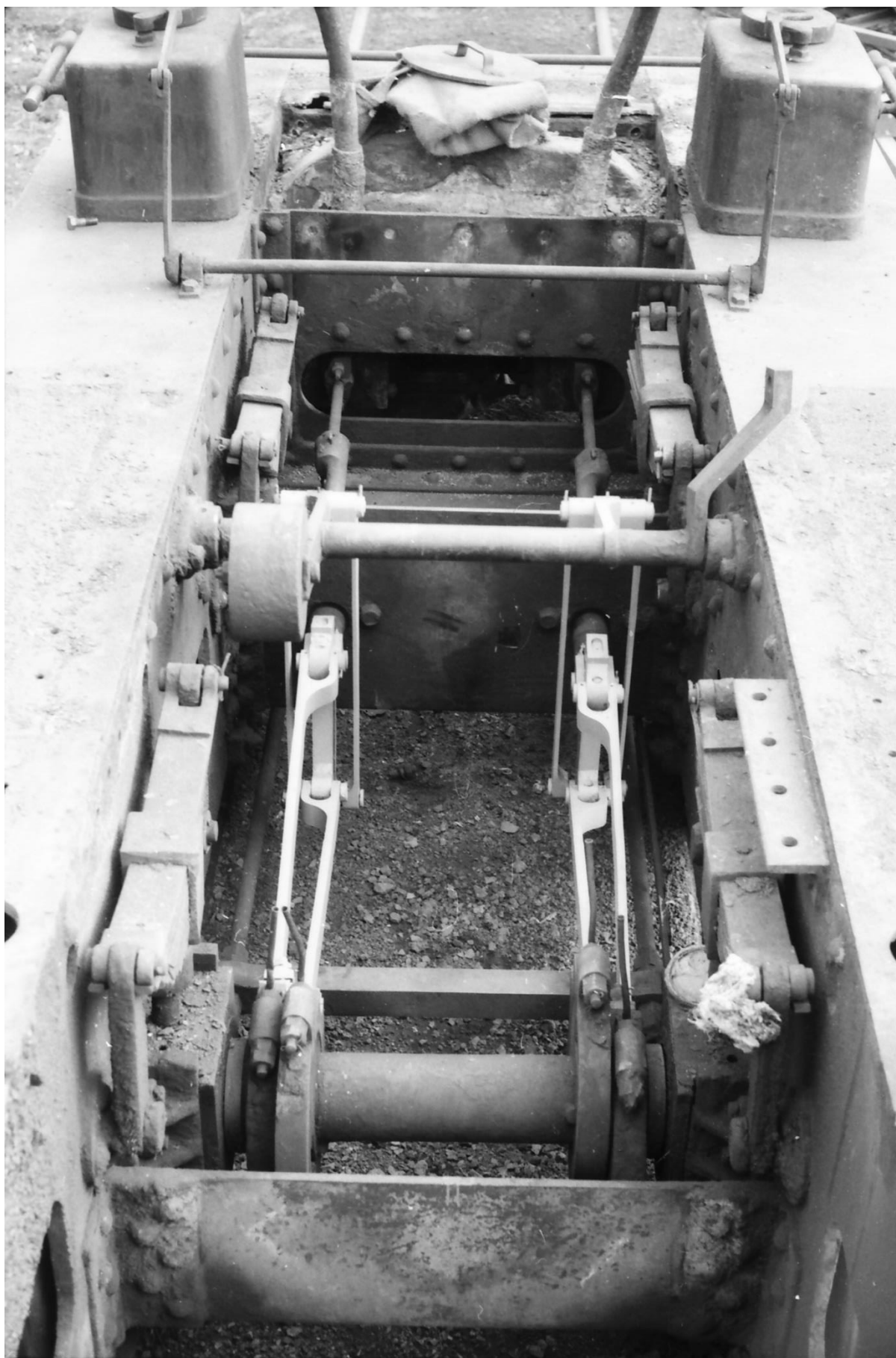
The Stephenson's valve gear showing fresh paint on the Peckett chassis circa 1970 (R.J.Mann)
