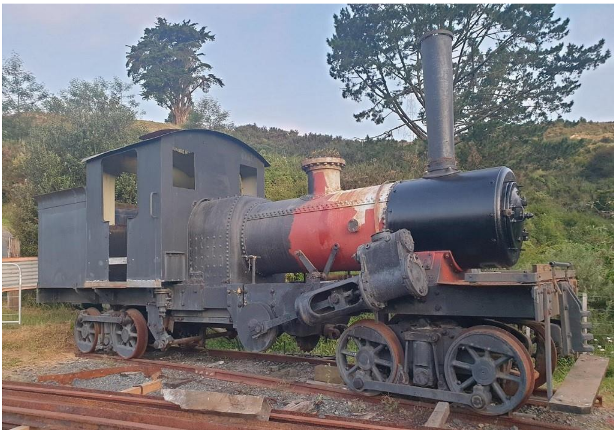
Work progresses on the Price "E" as a static exhibit. New smokebox etc. by R. Stratford (I. Jenner)
