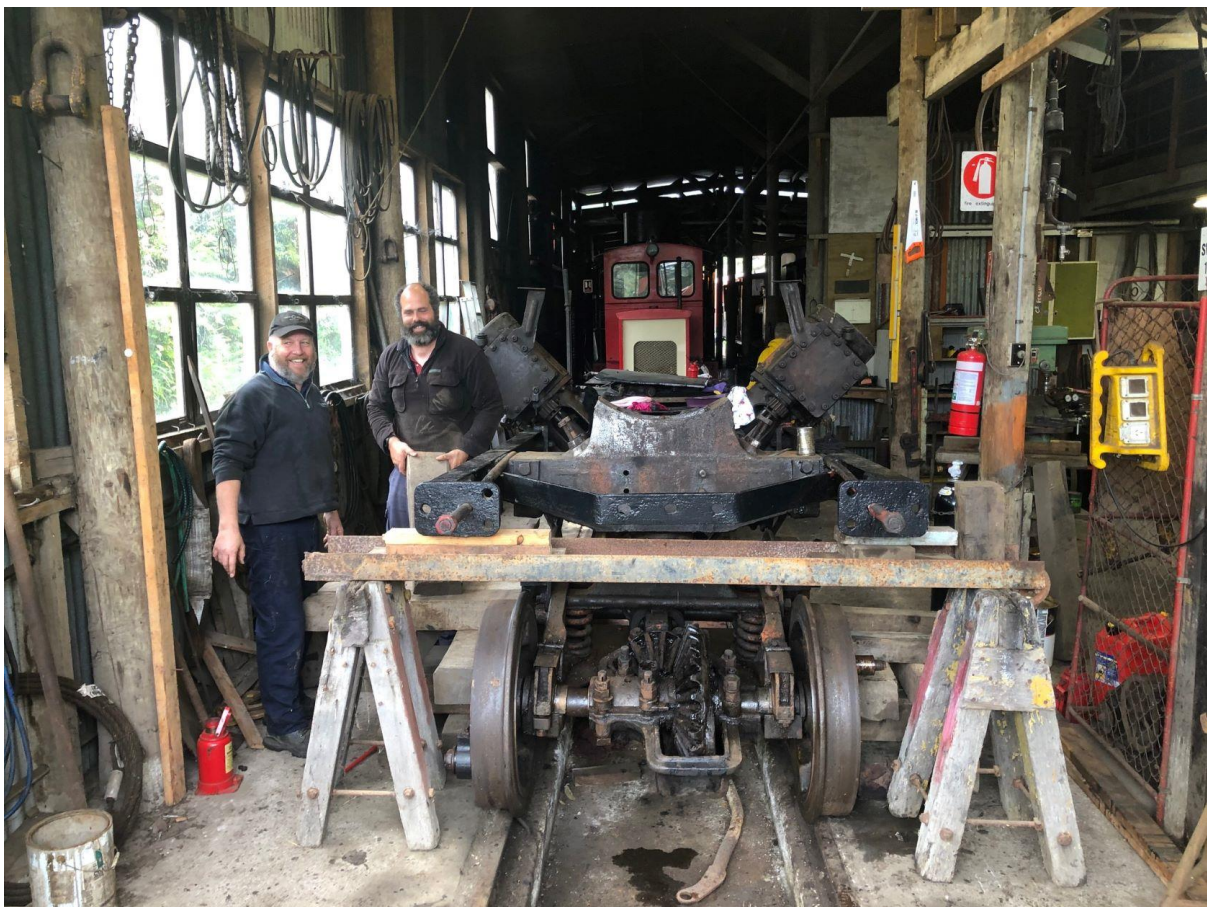
Pete C and Ian W in the loco shed are working on the Heisler bogie (C.Mann)
