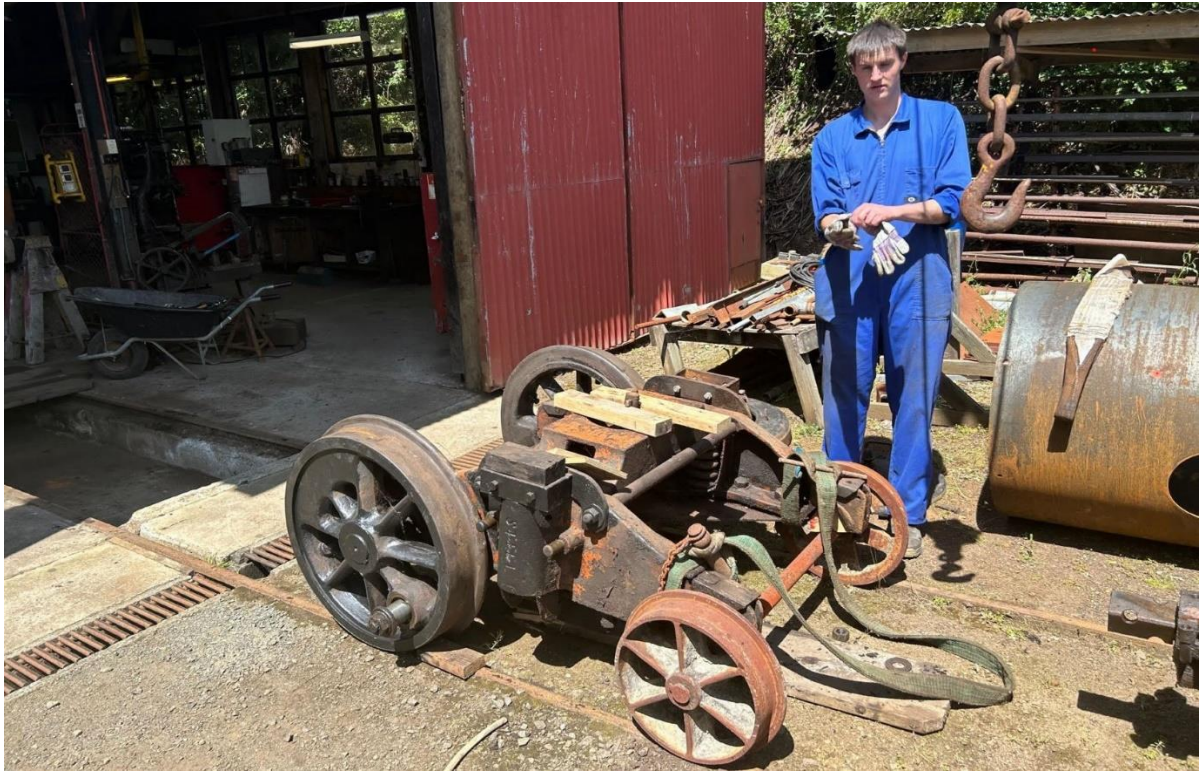
New volunteer Fraser R has been working on the Heisler – here we see a temporary wheelset keeping the bogie “on the rails” (C. Mann)
