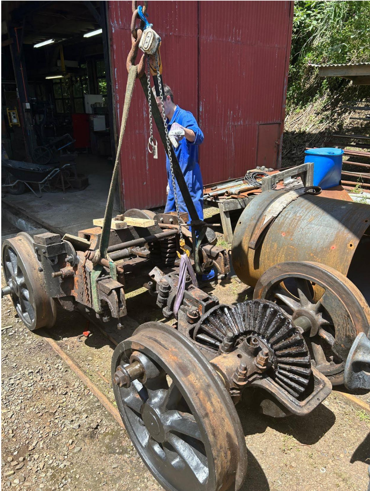
The Heisler bogie frame is hoisted at one end to remove a wheelset (C.Mann)
