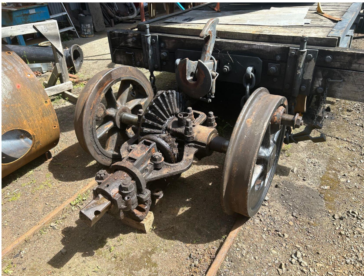
A wheelset from the Heisler shows the bevel gear arrangement (Photo: C. Mann)
