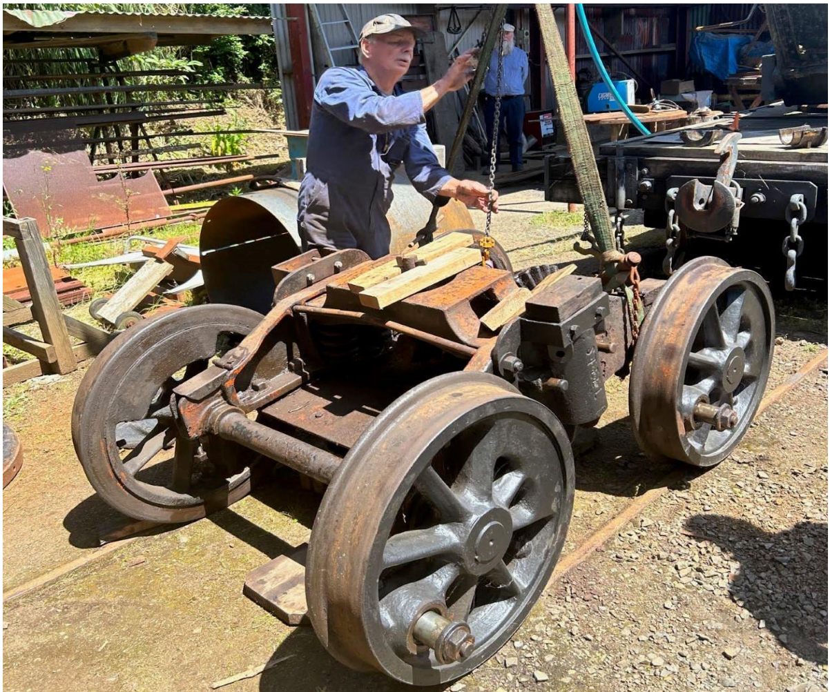
Richard S in action with the Heisler bogie strip down (C. Mann)
