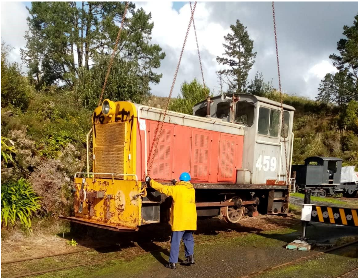
Tr459 is lowered by crane onto the BTC track (R. Webb)
