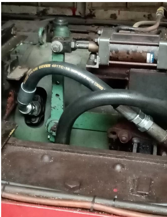
Tr105 has a new hydraulic hose on the torque converter (R. Webb)
