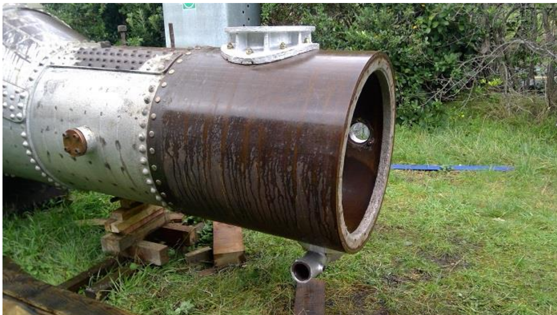
The new Heisler smokebox is now fitted (Alastair MacIver)
