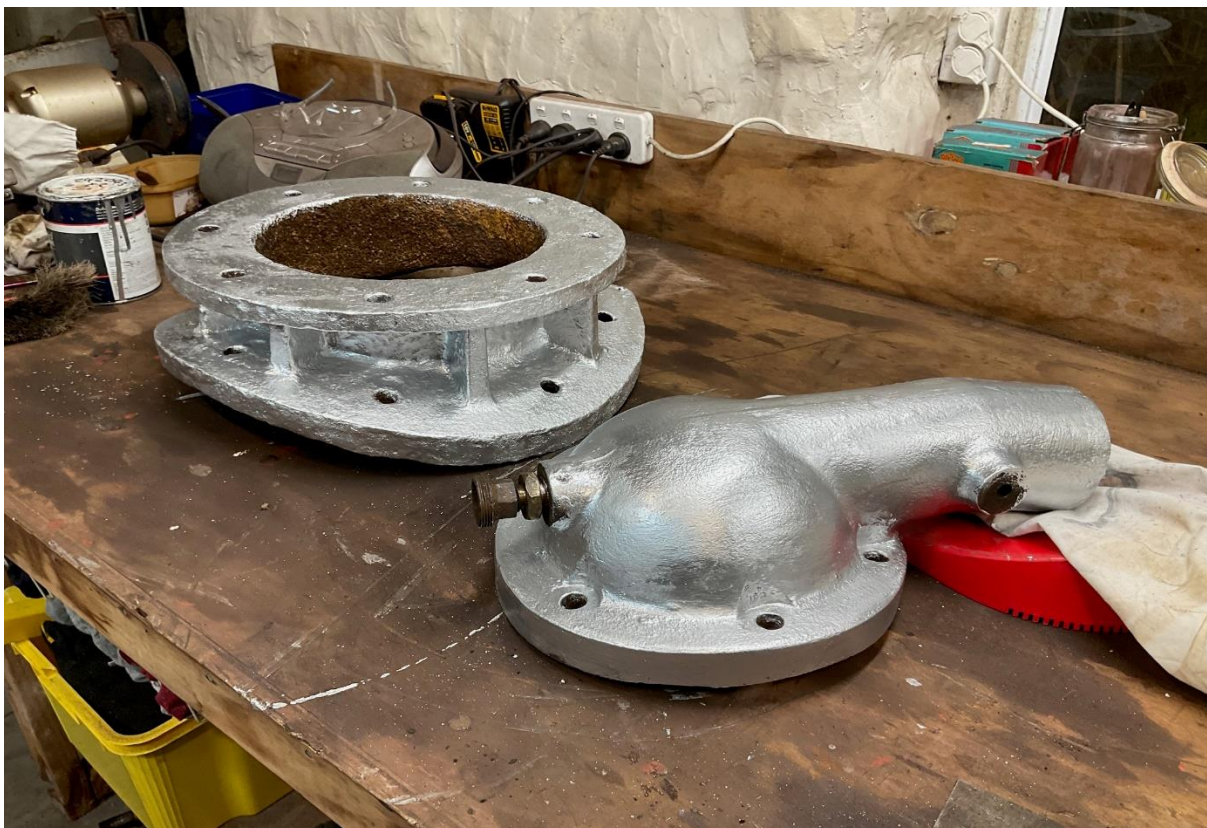
Above & next page (upper): smokebox componentry has been cleaned up for the Heisler project & shipped off to Paekakariki to be installed on the new Heisler smokebox (Chris Mann)
