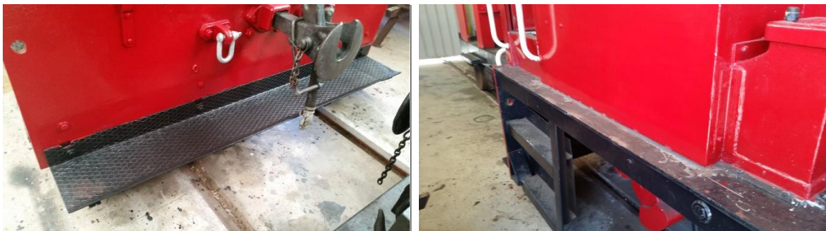
Tr 105 (Tr367) has recently had its rear shunter's footplate & cabside repaired (Images: R. Beaumont)
