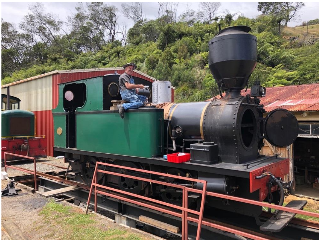
Dave Mann working on re-assembling the Peckett after its recent boiler survey (Image: C. Mann)
