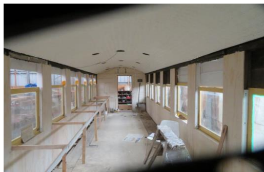
The interior of our A1477 "A" Class carriage is being lined with plywood prior to painting (Image R. Ellis)
