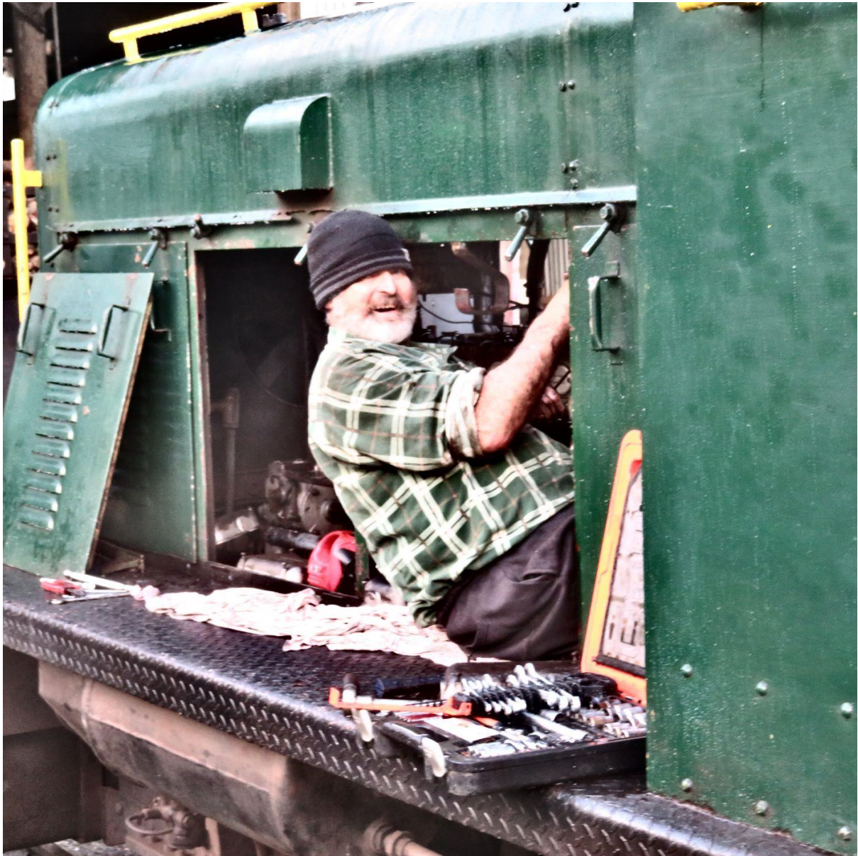
Geoff Boyle fits new injectors to 401's 8 cylinder Gardner engine (Image: R.Ellis)
