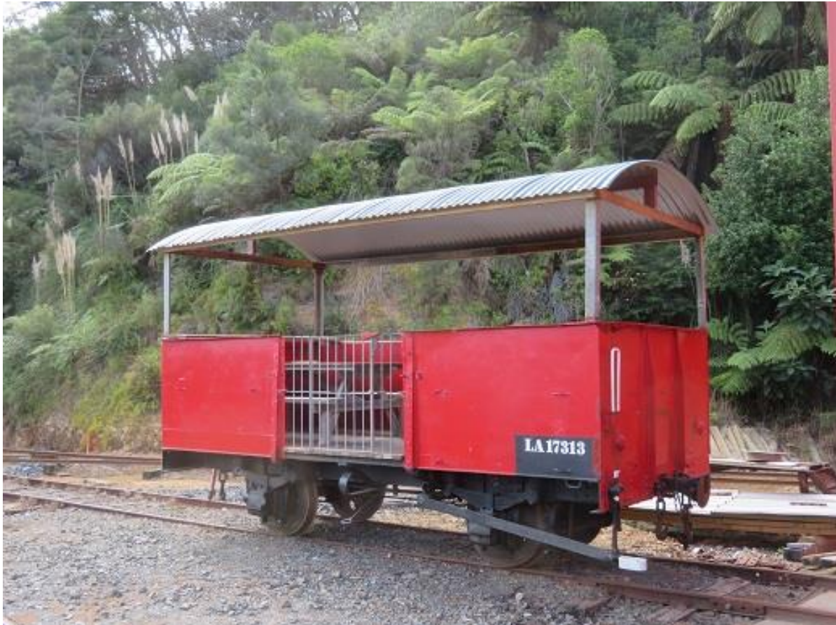
La wagon with its new roof (R. Ellis)
