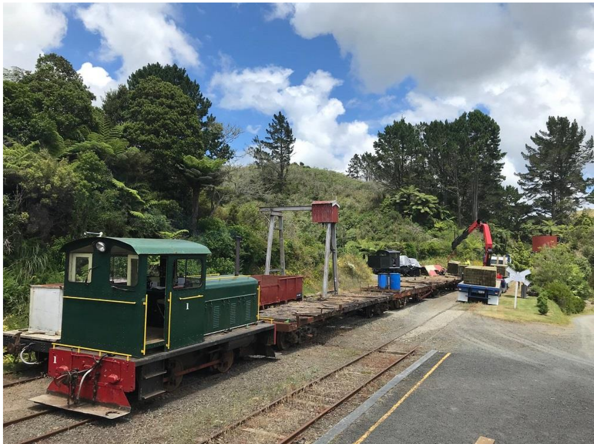
The Meremere diesel & flat wagons await the sleeper delivery to be transferred from truck to train...
