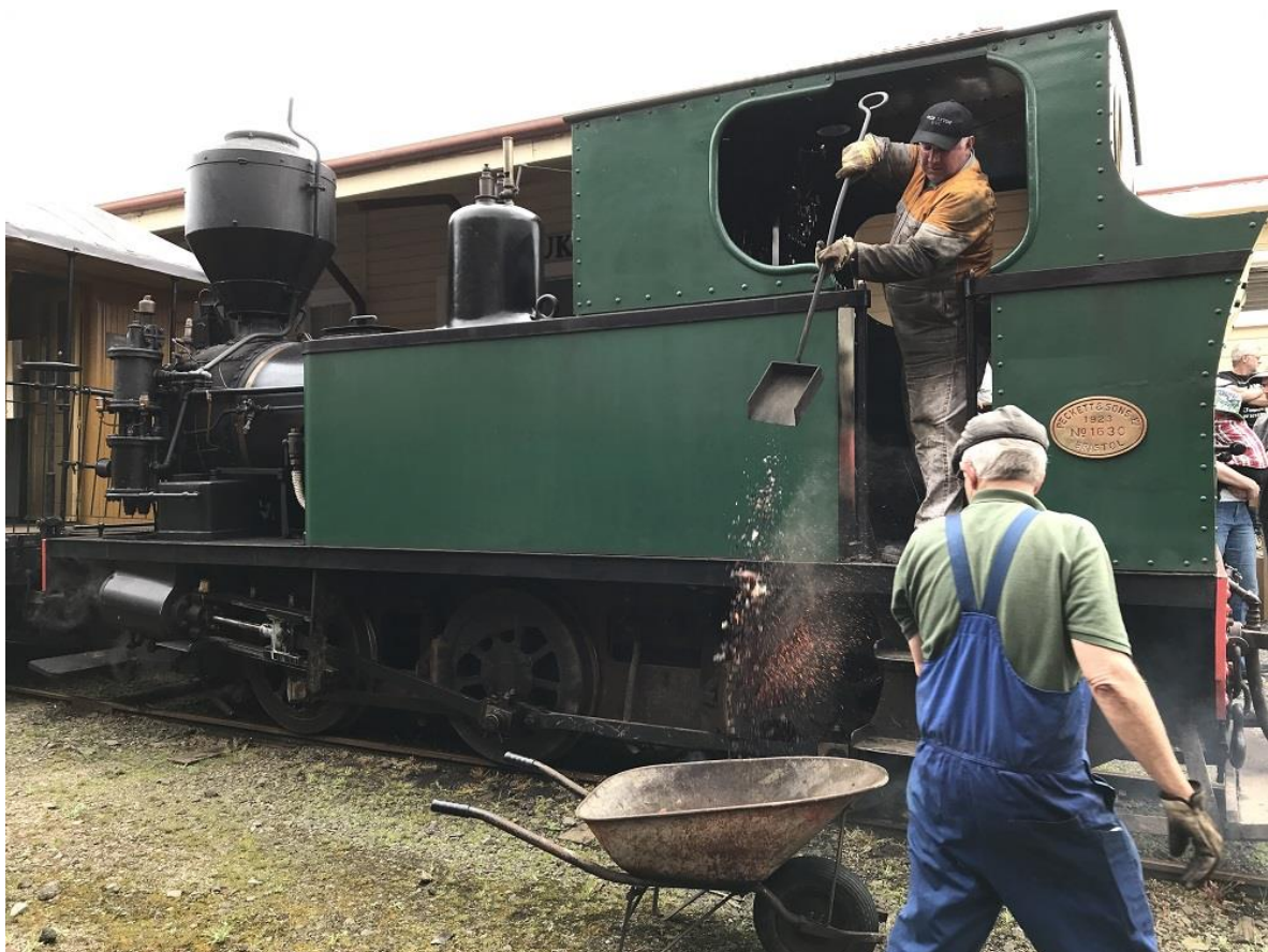
Neil Purdie & Bruce McLuckie hard at work ashing out the Peckett – note the red hot cinders!
