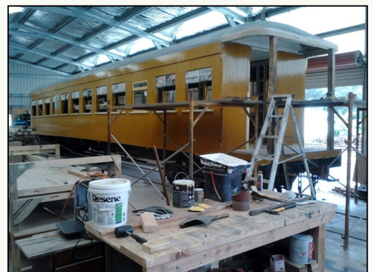
The main span of the new roof is Coloursteel with curvy balcony roofs of fiberglass (Images: R.E.)
