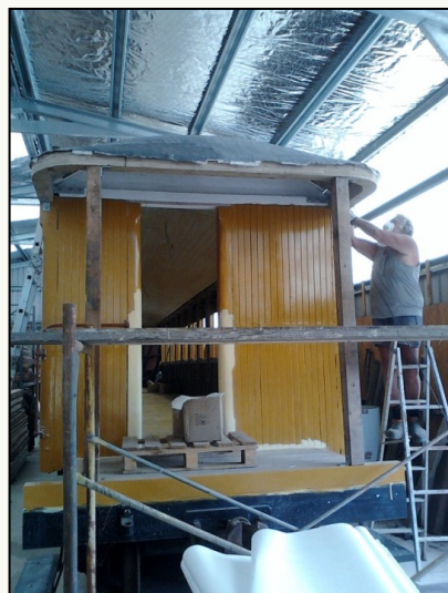
Surgeon Russell making "delicate adjustments" to the new fiberglass balcony roof which is bonded to beams fabricated by member Peter Cairncross. A better ladder would be appreciated (Image: R.E.)
