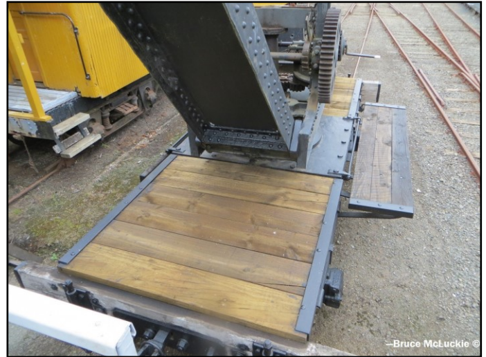
The new deck on the hand crane. I'm not sure if it will match the original deck well enough to be recast in any more 'The Last Samurai' films!
