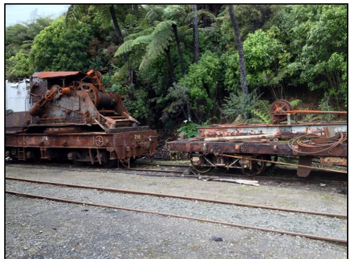
After a long search for a new home, the hard decision has been made to dismantle the club's steam crane for scrap. Here you can see the arm has been gas cut at the base and is now resting on its runner wagon
